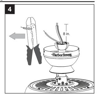
5. If you decided to cut back the lead wire in Step 4, strip 1/2 in. of insulation from the end of the white wire. Twist the stripped ends of each strand of wire within the insulation with pliers (not included). Repeat this step for black wire.
