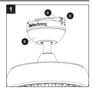
Secure the canopy (E) with the mounting bracket screws (G) previously removed (Step 4, page 8). Tighten all mounting bracket screws (G) securely.
