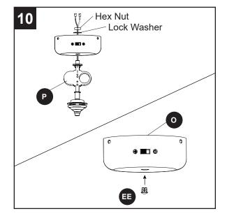
11. Remove the three fitter plate screws (M) from the fitter plate (L). Connect the 6-pin connectors from the fitter plate (L) and the light kit (P). Then, attach the switch housing (O) to the fitter plate (L) using the fitter plate screws (M).
