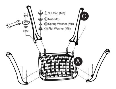
Step:2 Attach Back (B) to Seat(A) with Flat Washers(Part #2), Spring Washers(Part #10) & Nuts(Part #4). Note - Do not tighten Nuts(Part #4) completely at this time.
