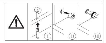
Cover No.1 plate to the top of the unit, and turn cam lock(E) in No.2,3,4 plates clockwise to tighten as shown.
