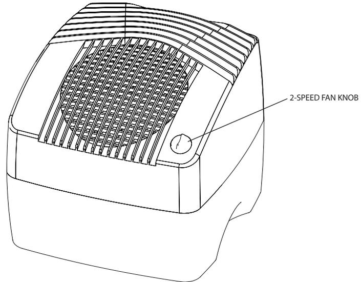
1) This unit has two fan speeds controlled by the lower right hand knob.
