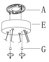
4 » Carefully pass supply wires through mounting plate (A). Secure mounting plate (A) to the outlet box with mounting screws (D).
