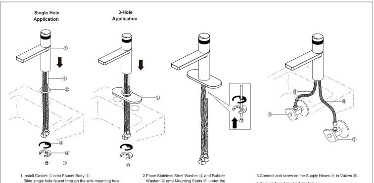
sink, and tighten the Mounting Nuts (5) securely
