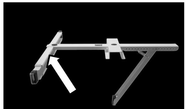
6. Now place the support bracket in the window. Push the leg out so it will rest snugly against the exterior of the house. The interior crossbar should be against the wall, framing, or the window trim. **DO NOT REST AGAINST THE WINDOW FRAME**
