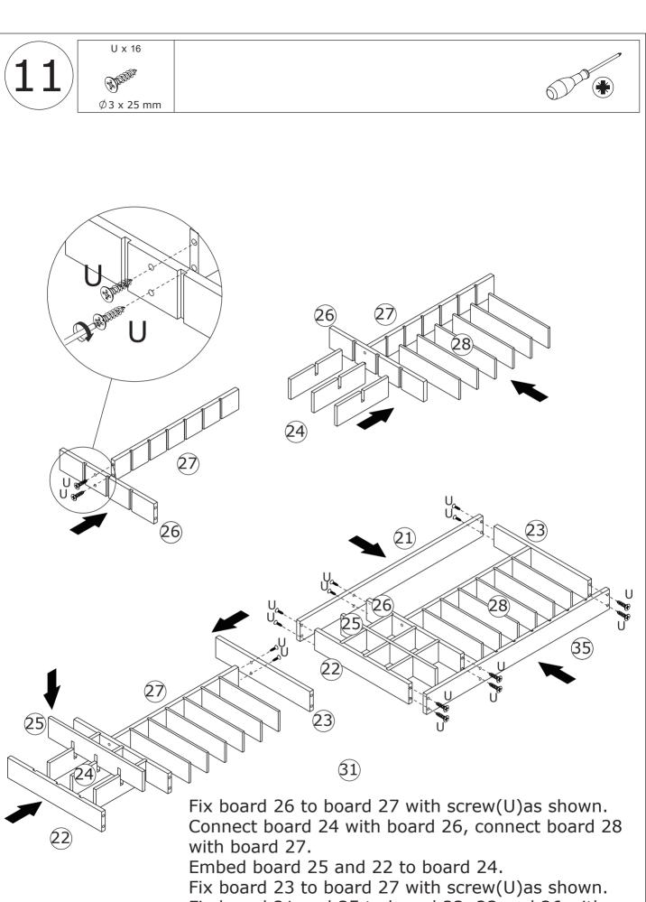
Fix board 23 to board 27 with screw(U)as shown. Fix board 21 and 35 to board 22, 23 and 26 with screw(U)as shown.
