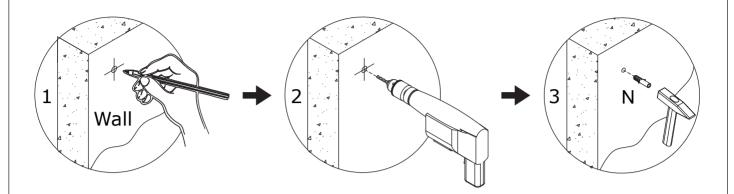
Install anti-tipping device as shown.
