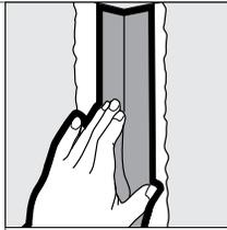
Next, fold joint tape along center crease and lightly press into position with your fingers.
