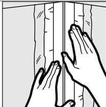
Press paper faced metal bead in place and embed by running a knife over each side with even pressure at a 45° angle.
