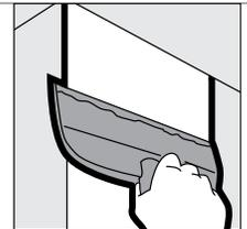
Allow first coat to dry overnight. Apply second coat of all purpose or topping joint compound with 8 in. knife, feathering slightly beyond first coat. Allow second coat to dry overnight. Sand lightly if necessary. Apply third coat with 10 in. knife, feathering slightly beyond second coat.
