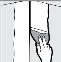
Using a 4 in. knife, apply an all purpose or taping compound to wallboard surfaces, extending compound just wider than the trim.
