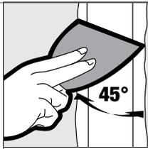
For best results, apply medium pressure and hold knife at a 45° angle to panel. Joint compound should be thinned slightly with water for easier application. For one gallon of compound, add water in 2 oz. increments.
