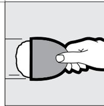
For each fastener depression, apply all purpose or topping compound horizontally with a 5 in. knife.
