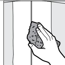
A damp sponge may be used to remove excess compound beyond the blade edge. Allow to dry.
