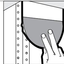
Apply all purpose or taping joint compound with 8 in. knife onto one flange, working down entire length. Hold knife at 45° angle and smooth compound. Compound should extend onto panel a minimum of 4 in. Repeat for other flange.
