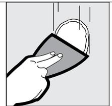
Next, raise knife blade to an upright position and wipe off excess with a right angle stroke. Compound should be level with panel surface. Allow to dry overnight. Scrape off bumps, ridges and other imperfections with knife. Be careful not to damage. Apply another coat to fasteners in same manner as first coat.
