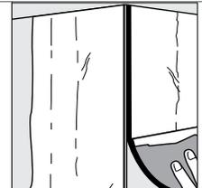
Using a 6 in. knife for outside corners (4 in. for inside corners), apply another coat of all purpose or topping compound. Keep this coat as smooth as possible, feathering out approximately 1 in. beyond previous coat. Let dry.
