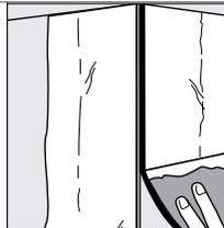
Once bead is in place, use a 4 in. knife to apply a thin layer of compound over the paper facing, while pressing out excess compound and eliminating air bubbles.
