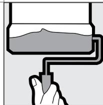
Prior to painting, apply USG Sheetrock® First Coat Primer or a flat latex paint.
