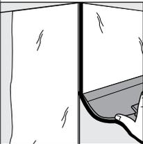
Lightly sand to remove high spots. Then use an 8 in. or larger knife for outside corners (4-6 in. knife for inside corners) to apply finishing coat, feathering approximately 2 in. beyond previous coat. Let dry; sand lightly.
