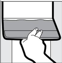
Allow joints' second coat to dry overnight. If necessary, remove imperfections with knife or sandpaper. Apply a thin finishing coat of all purpose or topping compound with a 10 in. or 12 in. knife. Press knife firmly so joint compound fills depressions but does not significantly add to thickness. Feather edges at least 2 in. beyond second coat. Allow third coat to dry overnight.
