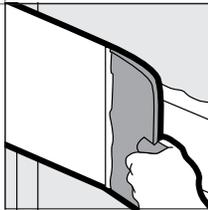
For tapered joints, apply all purpose or topping joint compound to the length of the joint using an 8 in. or 10 in. knife. Joint compound should extend 2 in. beyond first coat for a total width of 7 in. to 10 in.
