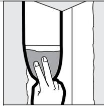
Allow first coat to dry overnight. Apply joint compound down length of one side using a 5 in. knife. Scrape off any compound that laps on to the second side. Feather out beyond first coat and allow to dry. After first side is dry, apply compound on other side, and feather.
