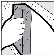
When only minimal sanding is needed, try wet sanding with a sponge. It eliminates dust and does not scuff the surface paper. Use a small-celled polyurethane sponge similar in appearance to carpet padding. Saturate sponge and wring to prevent dripping. Rub joints to remove high spots, using as few strokes as possible. Clean the sponge frequently during use.
