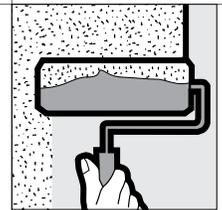
After prime coat is dry, apply USG Sheetrock® Wall and Ceiling Texture or a good quality interior paint.
