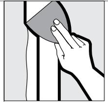
Center and lightly press in joint tape with fingers. Draw 6 in. knife firmly to tightly embed tape, but keep sufficient amount of joint compound beneath tape to prevent blistering.
