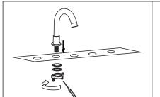
Make sure there are 5 mounting holes in the panel. (1)The main body is put into the hole 6 the following installation nut into 234, and the main body link.
