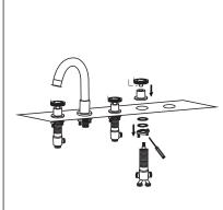
3. (9 2) The main body on the panel, (19) each (25) links installed, lock the main body with a hexagonal spoon (9, Tighten the nut again.
