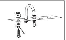
2. ⑤⑦ The main body on the panel, ⑤each ① links installed, lock the main body with a hexagonal spoon (5), Tighten the nut again.
