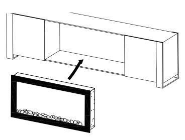
D: Push the fireplace into the mantel, and then fix the fireplace to the mantel with three screws from the back.
