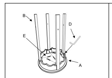
Step 1: Take all packaging off the table. Screw legs B 4pcs to table top. 4pcs screws E required. Allen key driver D required.
