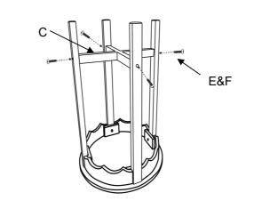
Step 2: Screw the X cross wood C to legs B. 4pc screw E & Allen key driver required. 4pcs wooden plug F to cork the screw holes.
