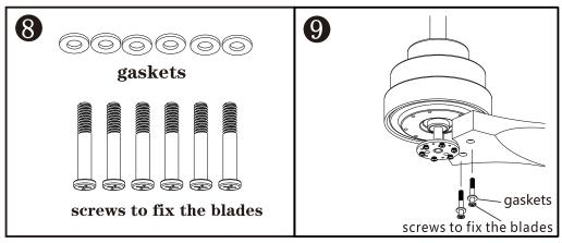
Note: The solid wood fan blades have a certain squeezing space. The blades must be installed with gaskets, and pay attention to locking with conventional force. Do not continue to apply force after the blades are locked to continue screwing in the screws, otherwise It will cause irreversible failures to the motor coil!
