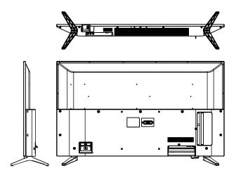
This Westinghouse TV is compatible with a 200mm x 200mm mounting hole pattern.
