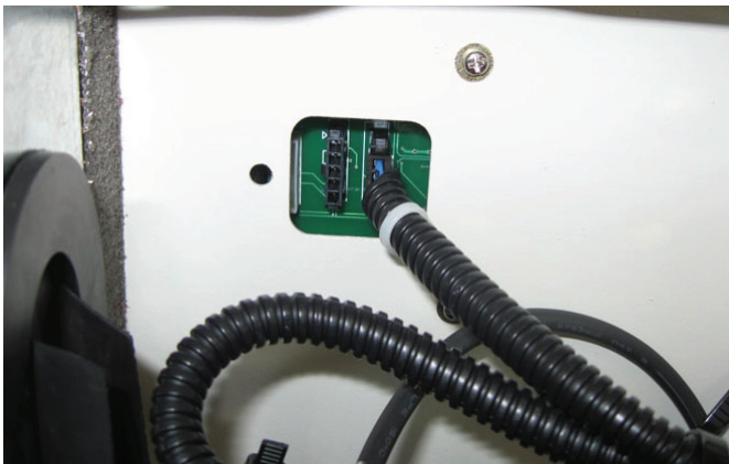
Figure 5 - Plug the 4-pin Plug into the Generator Transceiver Module
