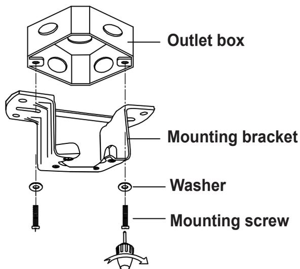
**WARNING: SHUT POWER OFF AT FUSE OR CIRCUIT BREAKER**
