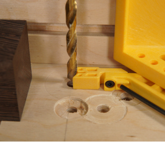
Fig 7b - P6 centering drill bit.
