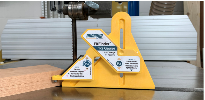
Fig 8c - P7 finding center on band saw.
