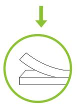
Tear off the double-sided tape of the light strip and stick it on the board.
