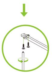
Hold the light strip with the clip and lock the screw.
