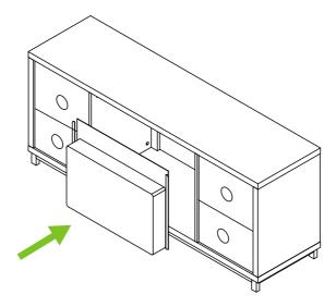
2 1Unscrew the two silver screws at the bottom of the fireplace 2. Then connect the iron sheet to the fireplace and the cabinet according to the corresponding hole position.
