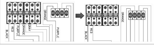
Figure 5 - Converting from Simultaneous to Non-Simultaneous Operation
