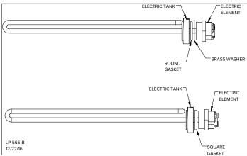
Figure 12 - Heating Element Detail
