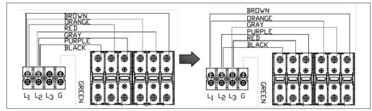
Figure 4 - Converting from Single to 3 Phase Operation
