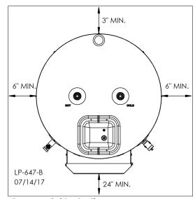
Figure 1 - Recommended Service Clearances
