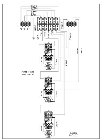
Figure 8 - 3 Phase, Simultaneous Operation
