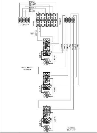
Figure 10 - 3 Phase, Non-Simultaneous Operation
