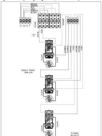
Figure 9 - Factory Wiring - Single Phase, Non-Simultaneous Operation
