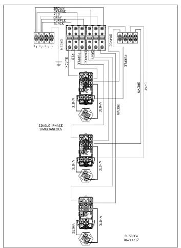
Figure 7 - Factory Wiring - Single Phase, Simultaneous Operation
