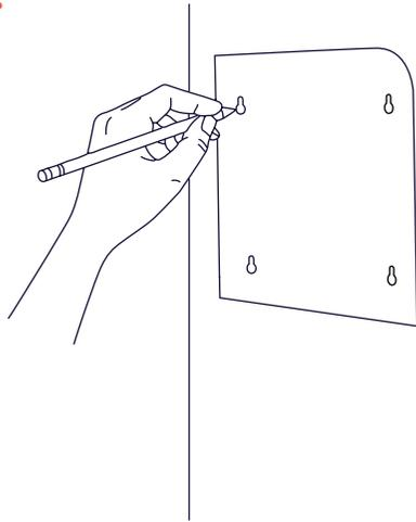
Position mounting template on the wall at the desired location. Make sure the unit is level and mark the drill holes.
