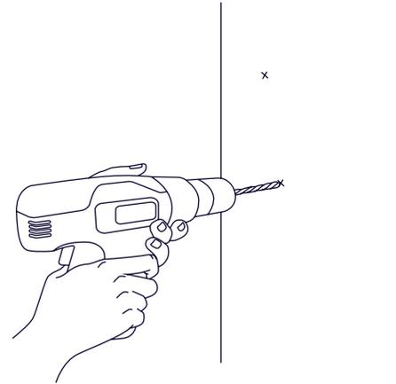
Remove mounting template. If mounting on drywall, use a 1/2" bit to drill pilot holes where the markings were made.
