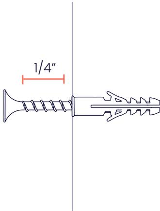
Use (4) drywall anchors and (4) mounting screws. Insert the anchors into the drilled holes, then thread screws into anchors. Do not thread screws all the way down. Leave them out about 1/4".
