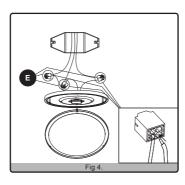
Place the fixture pan (A) over the pre-installed mounting screws and the mounting screws should align with two of the screw holes.
