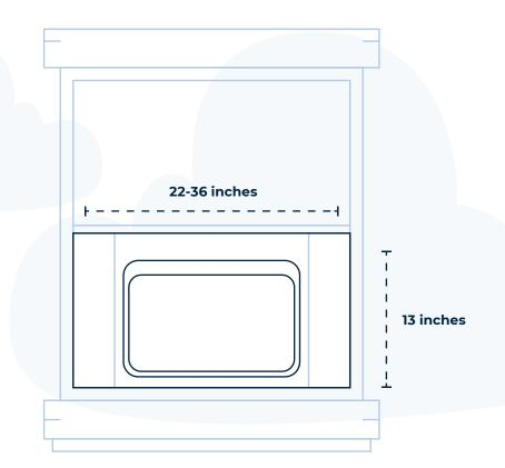
The small size (6K BTU) Windmill AC is designed for windows that slide up and down (double-hung windows) with a width of 22-36 inches and a vertical opening of at least 13 inches.
