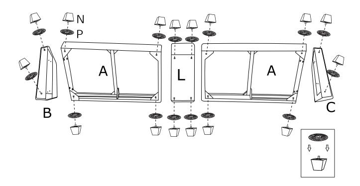
STEP 3: Assemble the Legs (N) on the Ottoman frame (H) with Gaskets (P) .
