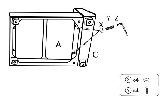
STEP 6: Assemble the Console (L) to the Seat frame (A) with Washers (X) and Blots (Y).
