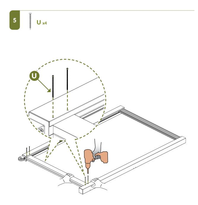
**Tip:** Ensure the bottom board is pushed to the back of the post channels before driving your screws.
