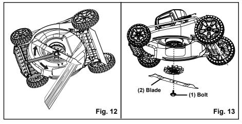
NOTE: Be sure to replace the parts in the exact order in which they were removed. When installing the cutting blade, verify that it is installed with the curved ends pointing toward the mower deck, and not toward the ground. Refer to the schematic drawing on page 32 of this manual.
