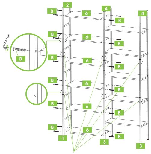
NOTE: The six holes must be on the same side when installing (with red "Back" mark).
