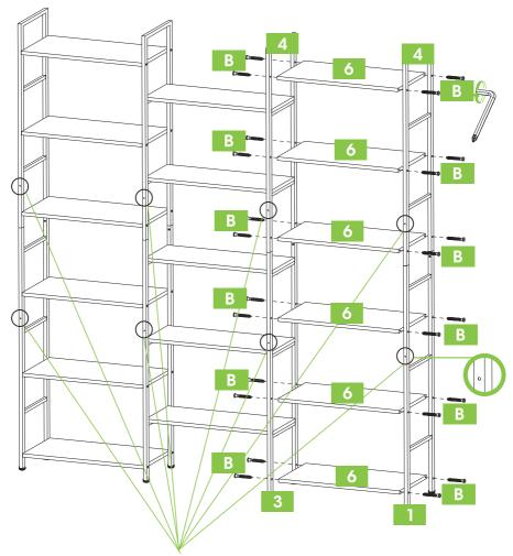
NOTE: The eight holes must be on the same side when installing (with red "Back" mark).
