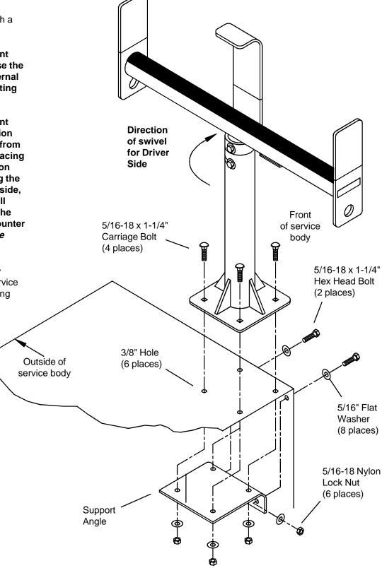
Figure 9. Front Stand Installation (shown on driver side)
