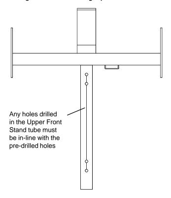
Figure 3. Hole alignment
