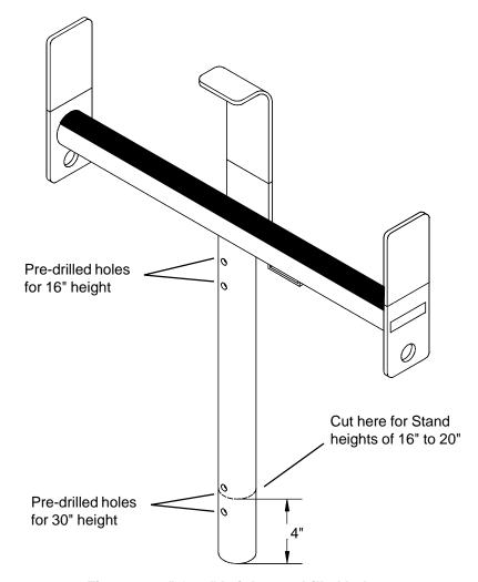
Figure 2. 16" & 30" height pre-drilled holes
