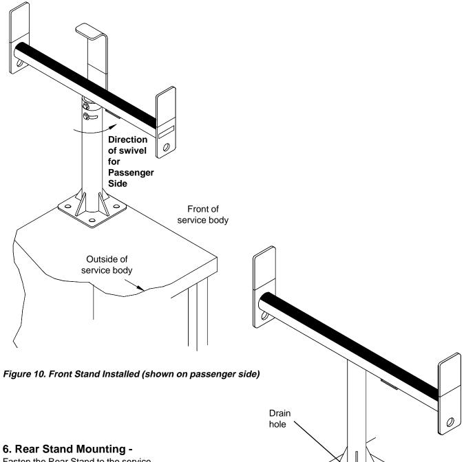
Fasten the Rear Stand to the service body with the upright tube drain hole towards the rear of the vehicle (See Figure 11.). The Rear Stand will fasten to the service body using the same fasteners shown in Figure 9..
