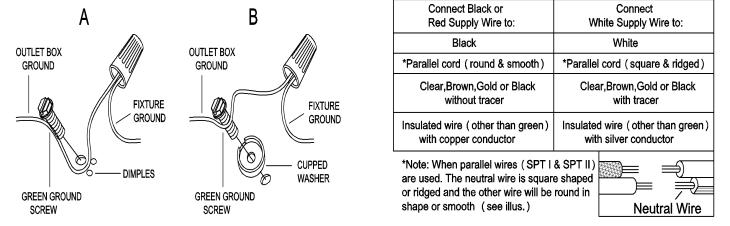
Twist plastic wire connector(A) until wires are tightly joined together, then carefully stuff all wires into the outlet box
