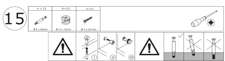
Insert quickfit screw(A) into No.21 plate as shown. Attach No.18 and No.19 to No.21 plate, turn cam
