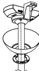
1. Carefully push the canopy to the bottom of the mounting bracket, make two sliding holes aligned to the two prominent screws on the mounting bracket, and then turn clockwise until tight.
