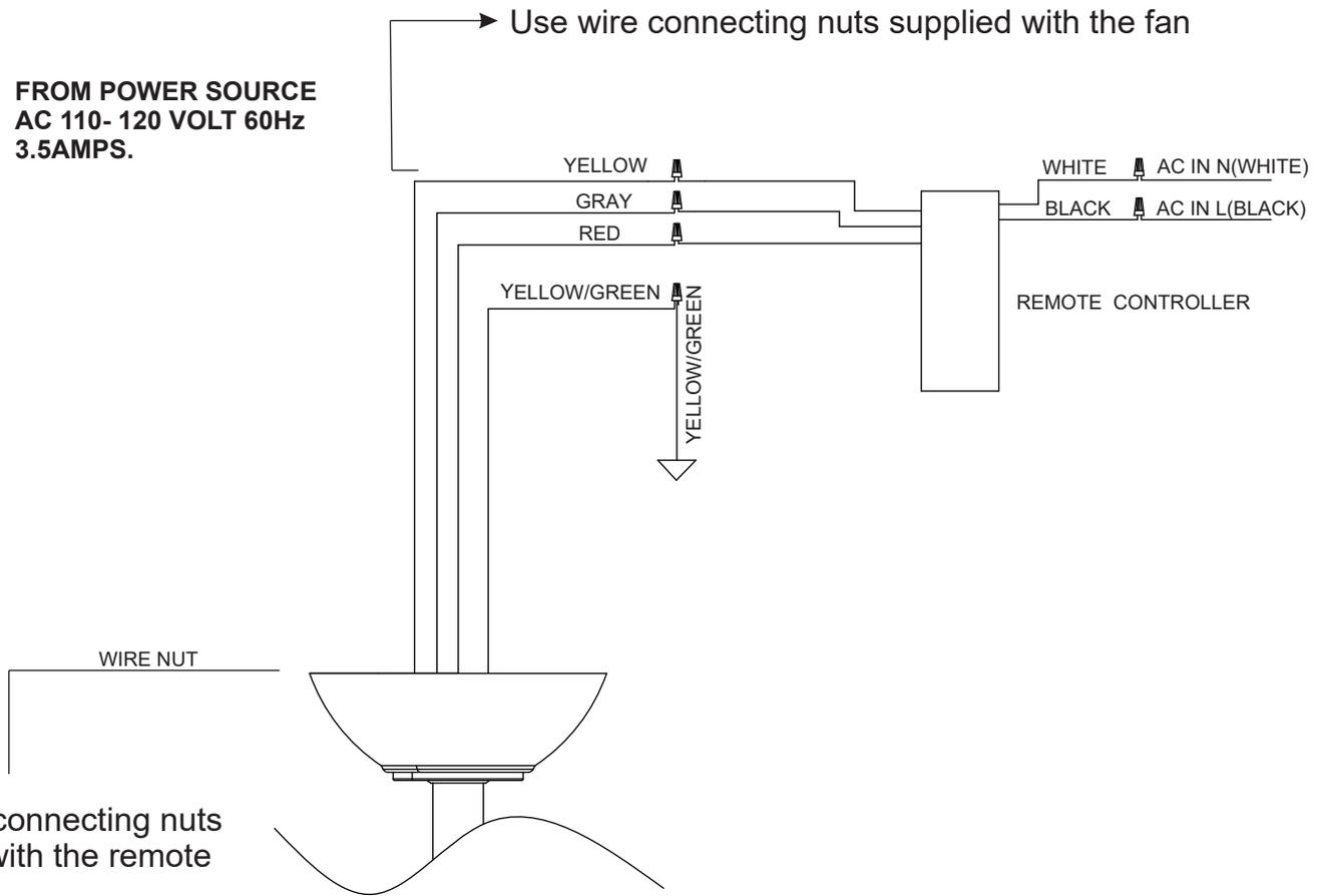
Use wire connecting nuts supplied with the remote controller.
