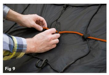
CAUTION: DO NOT HOOK ADDITIONAL ATTACHMENT STRAPS TO THE WEBBING LOOPS ON THE TARP; DAMAGE MAY RESULT. THE WEBBING LOOPS FUNCTION AS GUIDES FOR THE BUNGEES, NOT AS ATTACHMENT POINTS FOR ADDITIONAL STRAPS.
