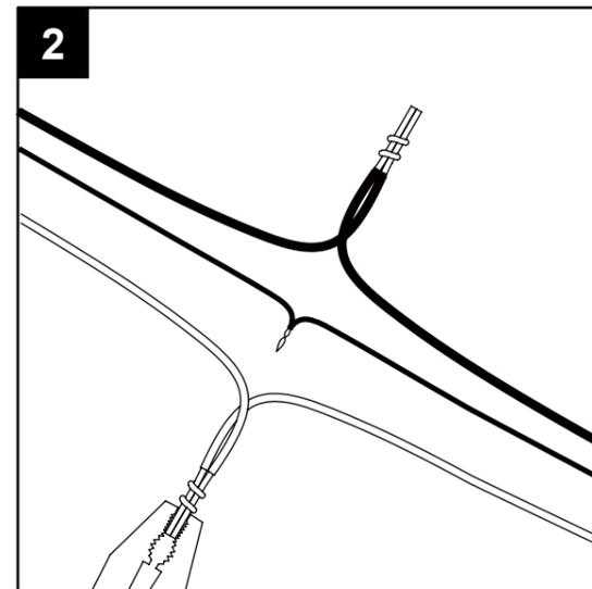
3. Attach wire nuts (BB). Tape wire nuts (BB) and wires together with electrical tape (not included).
