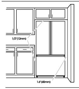
To ensure proper ventilation for your refrigerator, allow for a 1/2"(12mm) space on each side and at the top. Allow at least 2.0"(51mm) between back of cabinet and the wall. If your refrigerator has an ice maker, allow extra space at the back for the water line connections.
