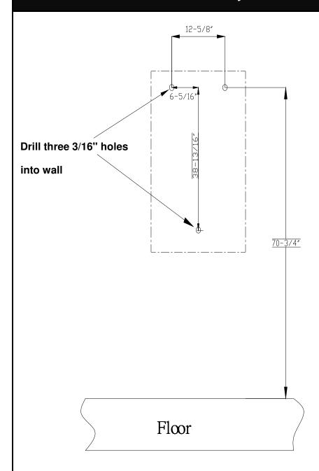
**Figure 1-Screw Hole Location**
