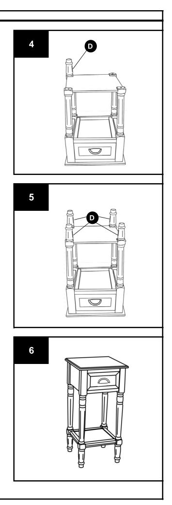
5. Slightly screw the other three feet through the bottom shelf to connect with the wooden legs.
