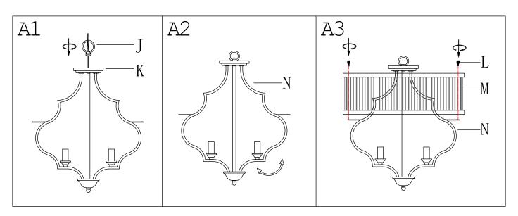
Step A1 » Screw loop (J) to the top of top assembly (K).
