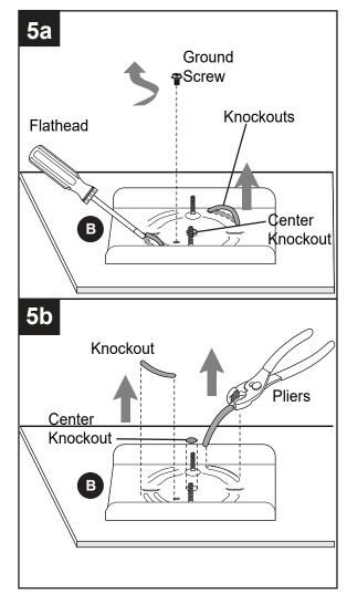
6. **IMPORTANT:** If you removed the ground screw in Step 5a, be sure to replace it before continuing.
