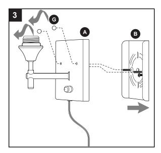
Remove mounting plate (B) from fixture (A) by removing decorative nuts (G) with fingers. Save decorative nuts (G) for later use.
