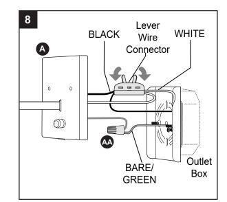
9. Wrap electrical tape (not included) around wire connector (AA) down to the wire.
