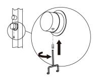
2 Thread metal lock-ring back on the valve
