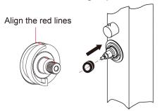
5 Use an allen wrench to tighten the HEX screw
