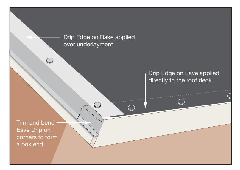
Begin installation along the eaves, starting at a corner and working your way around, overlapping each succeeding piece of drip edge by 2-3 inches.
