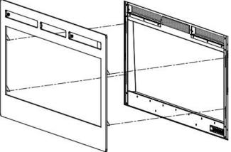
**4.A10)** Fix the glass front by screws (CC) and complete the installation.
