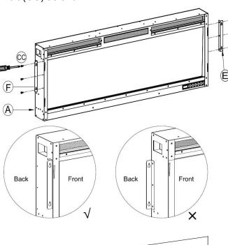
**4.A4)** Insert the firebox into the opening,
