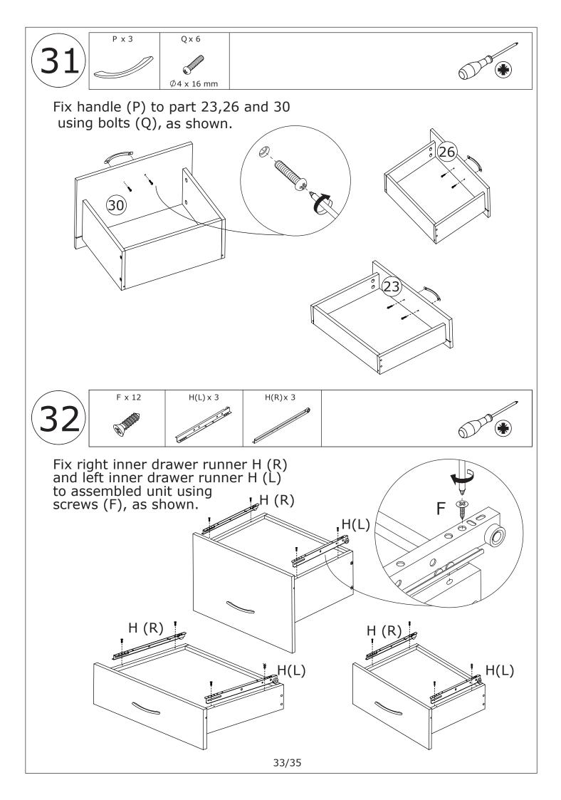
The drawer slides must be aligned with the internal rails, otherwise the drawer will tilt.
