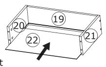
Slide part 25 into available slot of parts 20 and 21, as shown.
