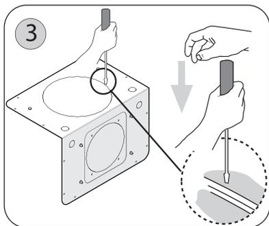
5. Install the flange and fix it to the blower plate with the (4) screws. Fig. 5
