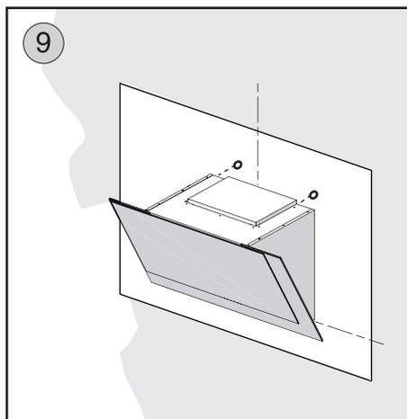
**NOTE1:** For the various installations use screws and screw anchors suited to the type of wall (minimum screw size: 1/4" diameter x 2-3/4" length).
