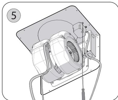
6. Secure Green/Yellow ground wire connected to the cable to the provided capacitor to blower plate. Fig.6
