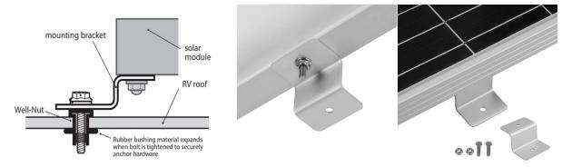
The solar panels can be permanently installed level using the Z-brackets.
