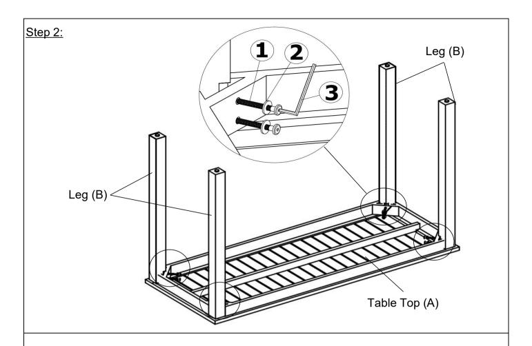
With the help of your adult partner, place the Table Top (A) facing down and then attach the Legs (B) to the Table Top (A) by using Bolt (1), Washer (2) and Allen Wrench (3). **Do not fully tighten the Bolts.**
