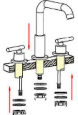
Place the faucet body and handles into sink holes, screw the plastic washer, metal washer and locking nut to the thread pipe of the faucet as photo 2
