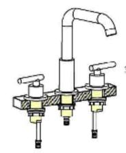
Adjust the position of the faucet and the handles then hand tighten the locking nut and then use a screwdriver to tighten the screws on the locking nuts to secure the faucet
