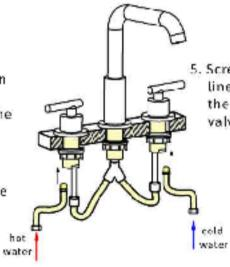
Screw the water supply lines to the faucet body, the handles and the stop valves
