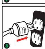
Plug in items to be powered, using only grounded extension cords
