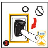
Run the generator at no load for 2 minutes and then turn engine switch to OFF (O) position
