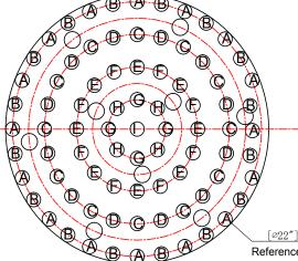
Reference for how to dress Note: Hang glass strand "A"and "B"alternating, "C" and "D" alternating, "E"and "F"alternating, "H"and "G"alternating.
