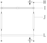
4. Screw tube (G) to canopy (E) and the top of sockets assembly (K) through upper iron frame (I). Hand tighten till snug.
