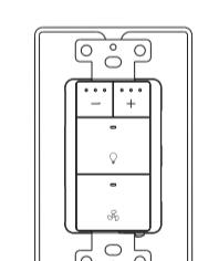
**Step 5:** If clear, place the radar sensor switch plate onto the switch and secure it with screws. Ensure the power prongs can slide into the electrical box.
