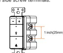
Remark: The distance between the L and L1 screws must be 25 mm for compatibility with the Radar Sensor Switch Plate.
