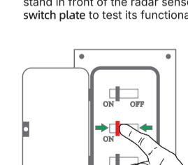
**Step 7:** The radar sensor switch plate is now installed. Please use the toggle switch on the device to customize the working time of LEDs after motion is no longer detected.
