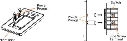
The power prongs slide around the side screw terminals and contact the lower screw heads to extract power for the Radar Sensor Switch Plate.
