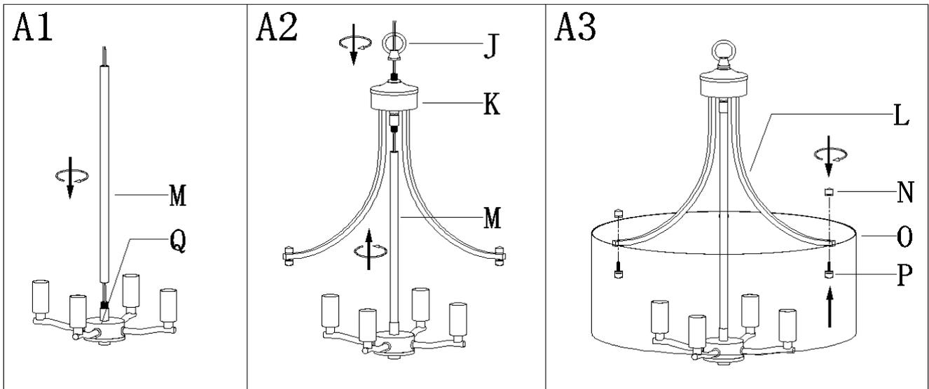
Step A1: Slip stem (M) over the wires and then thread it into the top of lower fixture loop assembly (Q).
