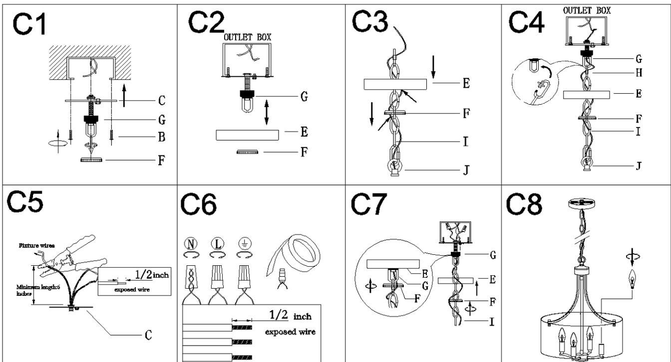
Step C1: Remove the collar ring (F) from collar loop(G). Attach the single bar (C) to outlet box with mounting screws (B). Be sure that the side of single bar marked "GND" must face out, then unscrew the collar ring (F) from the collar loop.
