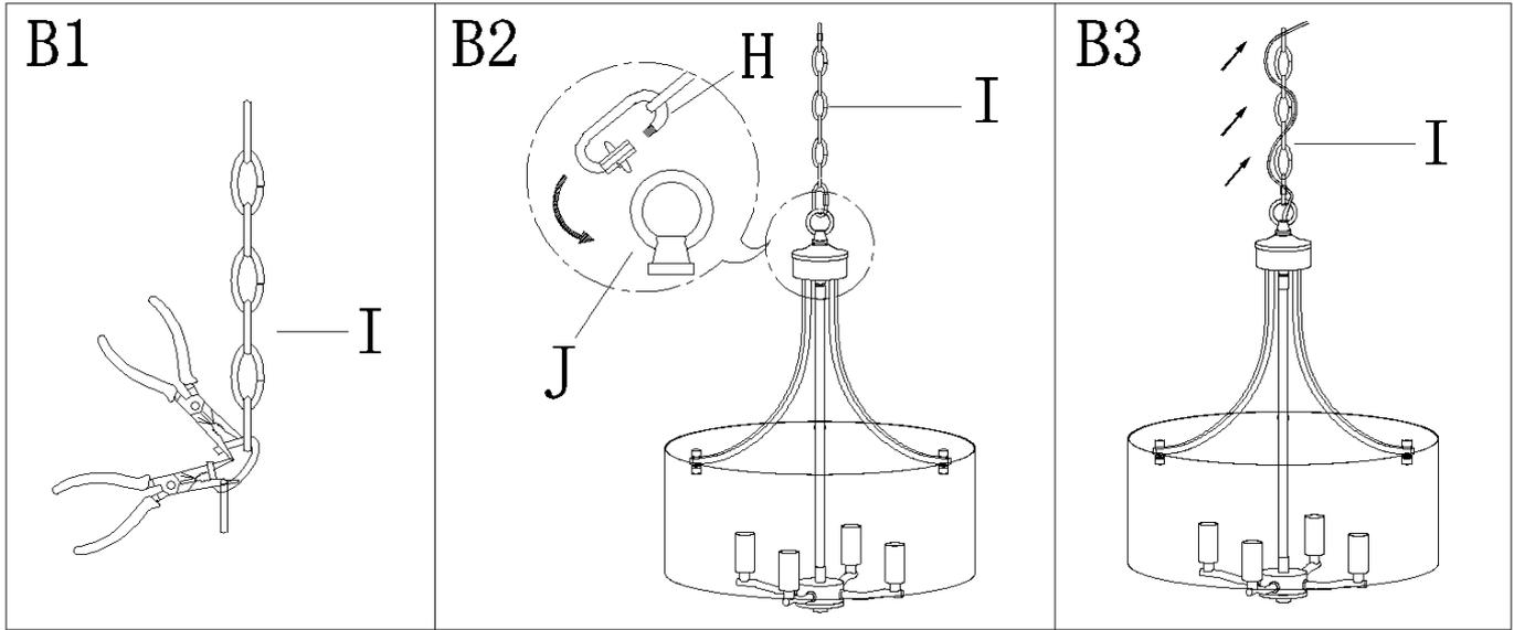
Step B1: By measuring, determine the correct number of links needed for proper hanging height. Using the chain pliers, disconnect and discard the unwanted part.
